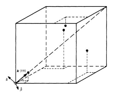
Crystal structure of B20 magnet (P2<sub>1</sub>3). There are four metal atoms in the positions (x, x, x), (x + 1/2, 1/2 - x, -x), (-x, x + 1/2, 1/2 - x) and  $(1/2 - x, -x, x + \frac{1}{2})$ . no inversion symmetry
