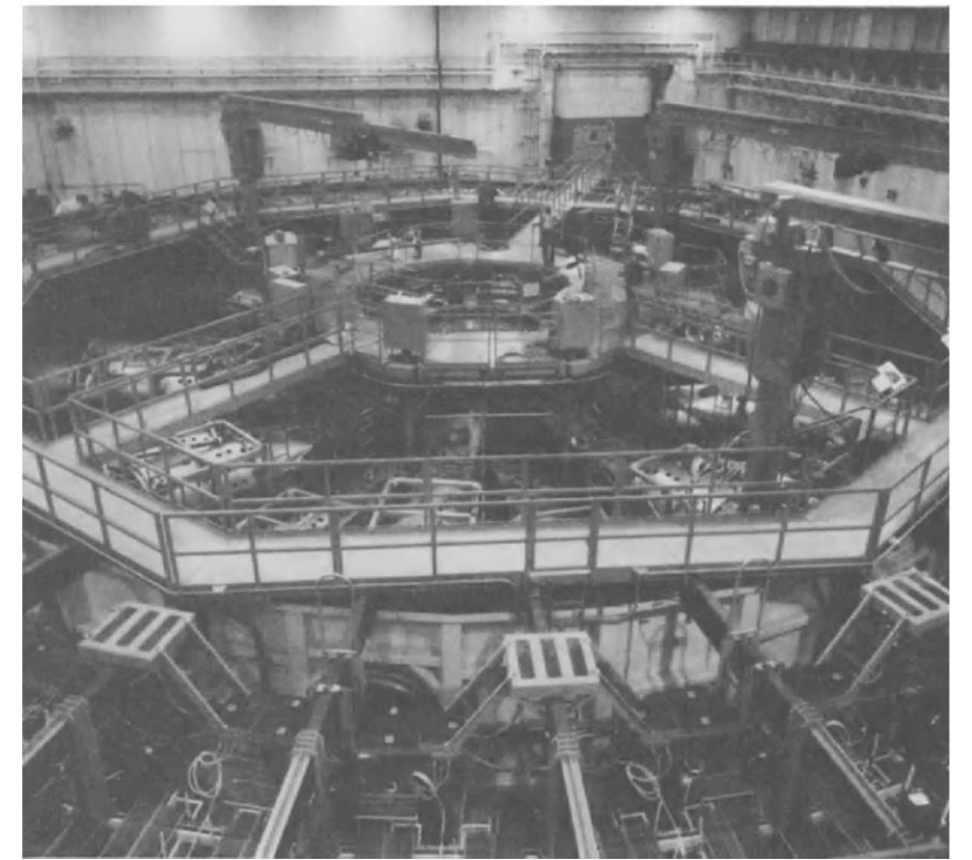
Figure 10-6. Nuclear fusion experiment at Sandia National Laboratories. Here, an accelerator focuses lithium ions onto deuterium-tritium pellets to produce nuclear fusion [VanDevender, 1985].
