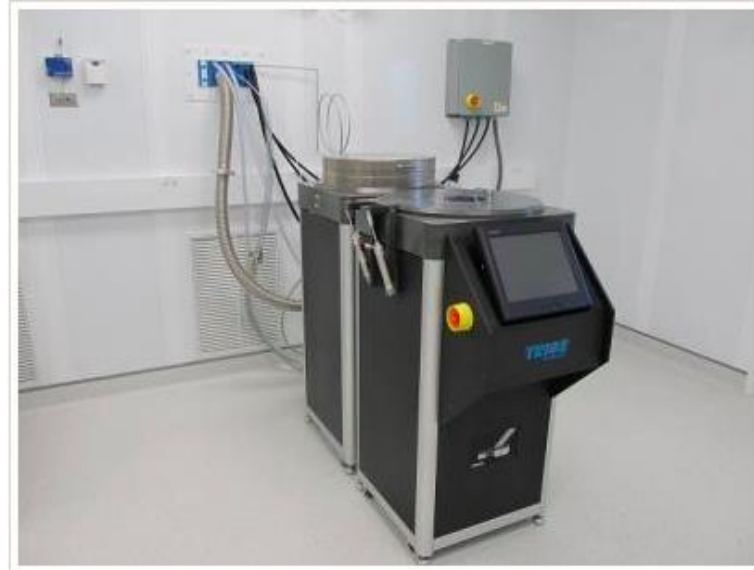
Reactive Ion Etching
